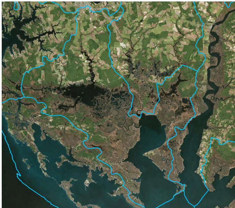
Figure 4-6. Example of HUC-10 local watershed boundaries superimposed on a map of Bay watersheds. Mapping of wetlands to model cells was restricted so as not to cross local watershed boundaries.
