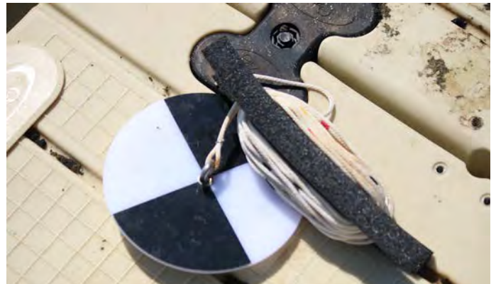
This Secchi disk is attached to a line that is marked with pre-measured distances. (Sky Swanson)
