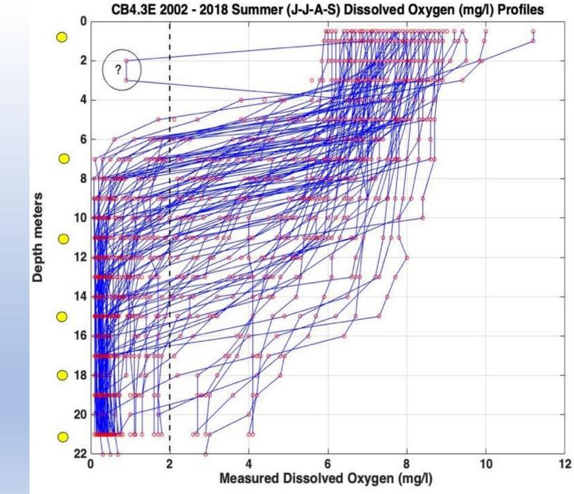
For station CB4.3E, reasonable results can be achieved with as few as five or six sensors graphical comparison of the sixsensor model is shown in Figure 1B. This is a preliminary analysis of sensor depths; it is likely that more rigorous placement analysis would reduce uncertainty even further.
