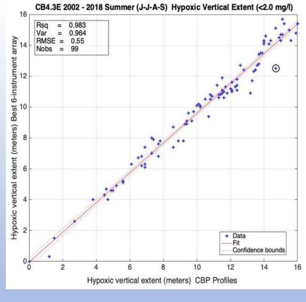
Comparison of 'Vertical Hypoxia Extent (Meters)' calculated using measured profiles (X axis) and the same quantity calculated using a hypothetical array of six sensors shown in previous figure. Different arrays were tested; the results are shown in Table.
