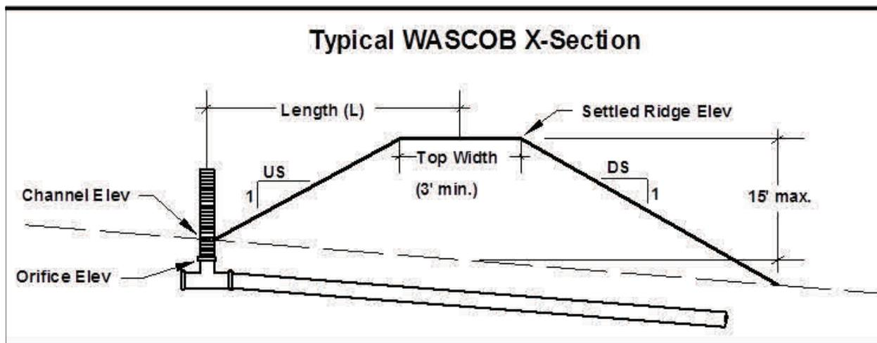
A water and sediment control basin, (WASCOB), is an earth embankment or a combination ridge and channel constructed across the slope of minor watercourses to form a sediment trap and water detention basin with a stable outlet.
