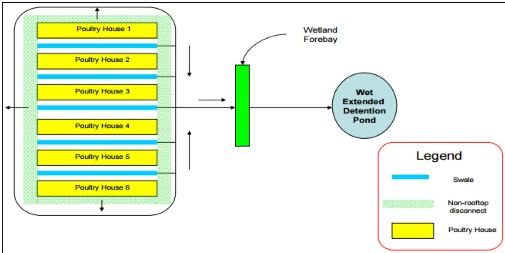
Figure 8. Current day model broiler farm with a wetland treatment system.
