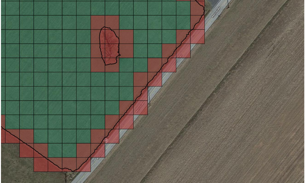
Figure 3. An example of identifying “mixed pixels” to exclude from remote sensing analyses. The thick black outline shows the original field delineation. This original delineation is crossed by several pixels (red) that have spectral responses that are combinations of the agricultural field’s spectral signature and other objects’ spectral signatures (e.g., those of the road and tree). Unless steps are taken to perform spectral unmixing, these mixed pixels should not be used for classification of the tillage regime. One method for removing these mixed pixels would be to erode (i.e., apply a negative buffer to) the original field delineation such that mixed pixels do not exist within the eroded polygon.
