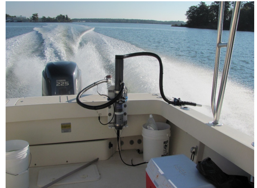
DataFlow measurement every 2 sec @ 25 knots \approx every 25 meters
