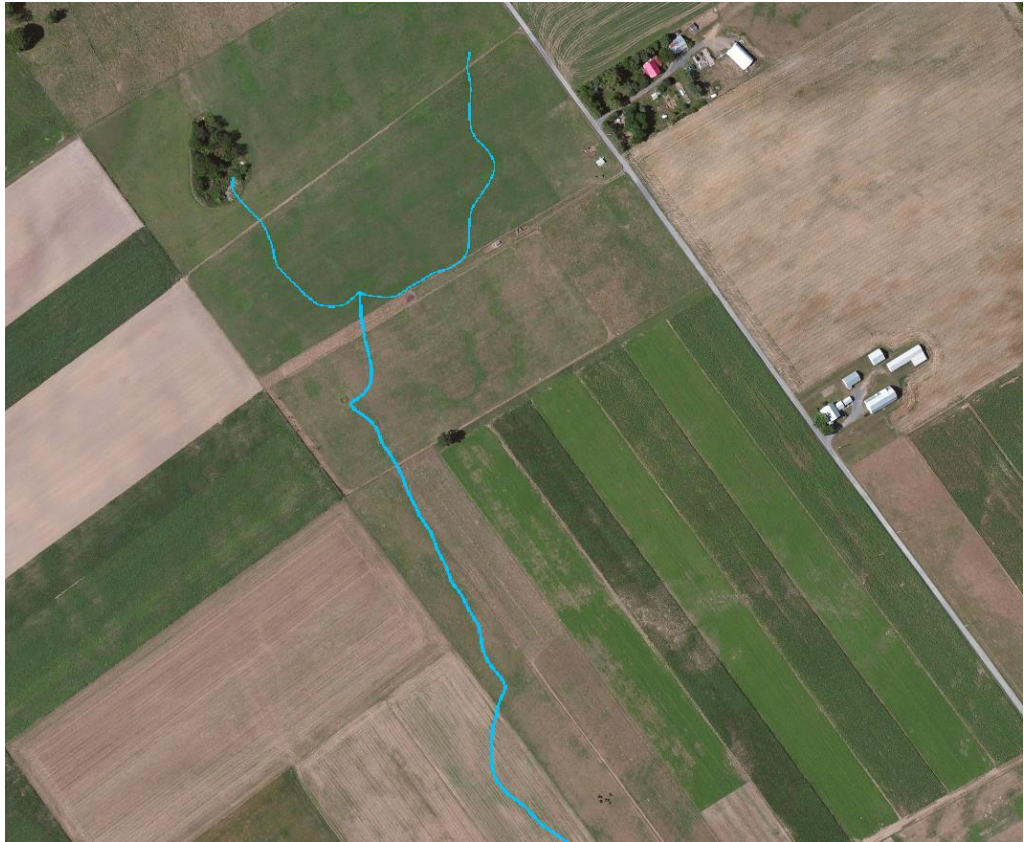
Example: False “stream channel” originating in a field as a result of 60 acre constant critical support area threshold
