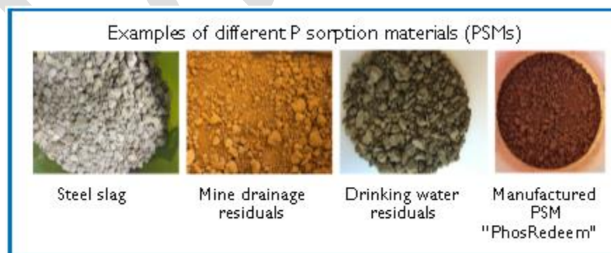
Figure 10. Examples of several P sorption materials (PSMs)
