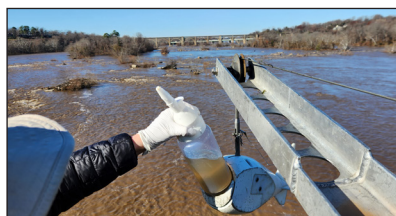
Individual collecting a nontidal monitoring network (NTN) water-quality sample.
