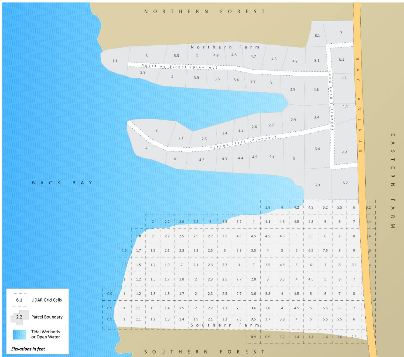
Figure 9. Example Scheme Showing Possibility of Reverter Based on Elevations for Two Large Parcels. In this example, the owner of the farm to the north has been working with a developer on a specific subdivision proposal. As lots are sold, the owner will retain a possibility of reverter, which she will transfer to The Land Conservancy. The reversion will be based on a different amount of sea level rise for each parcel, as shown in the platted lots. The owner of the farm to the south does not plan to sell during her lifetime, but she has agreed to sell a rolling easement in land for her farm as well. Without any specific subdivision plan, the southern farmer and TLC have agreed to base the reversion on elevations estimated by LIDAR. Thirty-meter grid cells are each assigned an elevation, based on the average of the three lowest 10-meter cells within the 30-meter cell. If the land is never subdivided, the transfer will take place cell by cell. If the farmer's children eventually subdivide the property, their developer will have to tailor lot boundaries and site plans to ensure that homes are entirely located within the part of a lot that reverts last. Alternatively, the children may propose another reversion scheme similar to that shown for the northern farm, which The Land Conservancy can accept if it is more beneficial to the environment than the LIDAR-based reversion shown here.
