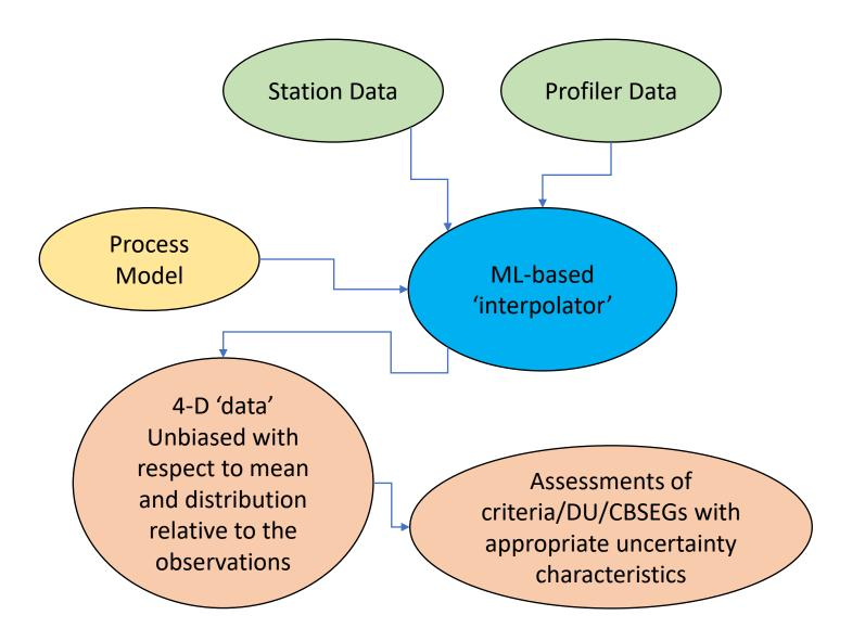
An 'interpolator', perhaps based on machine learning, would take inputs from station data, profiler data, and process models to produce a complete historical hourly record of DO on perhaps a 200x200x1 meter cell.
