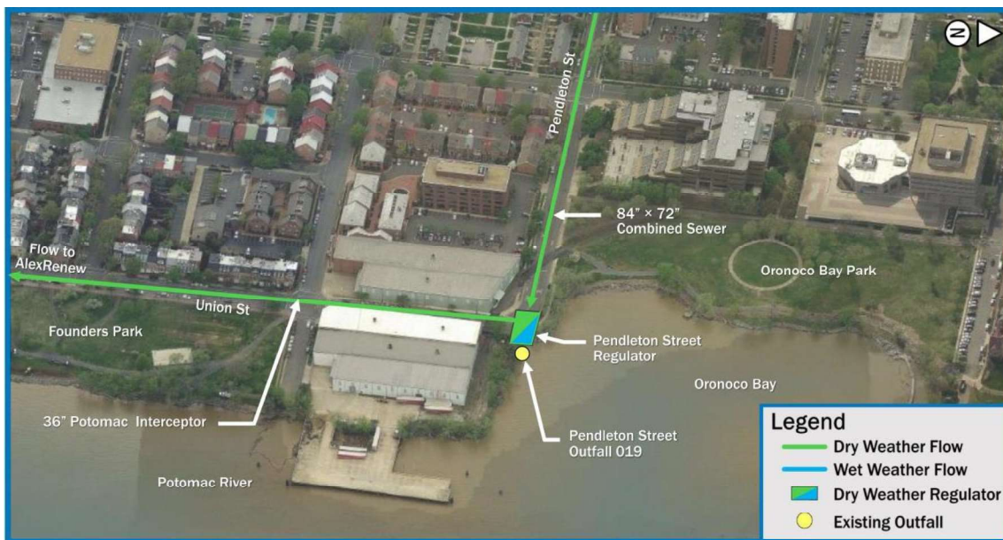
Figure 1-2. Pendleton Street Outfall 019 and Regulator
