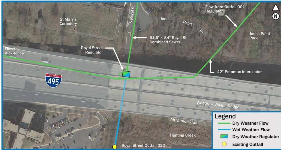
Figure 1-3. Royal Street Outfall 020 and Regulator
