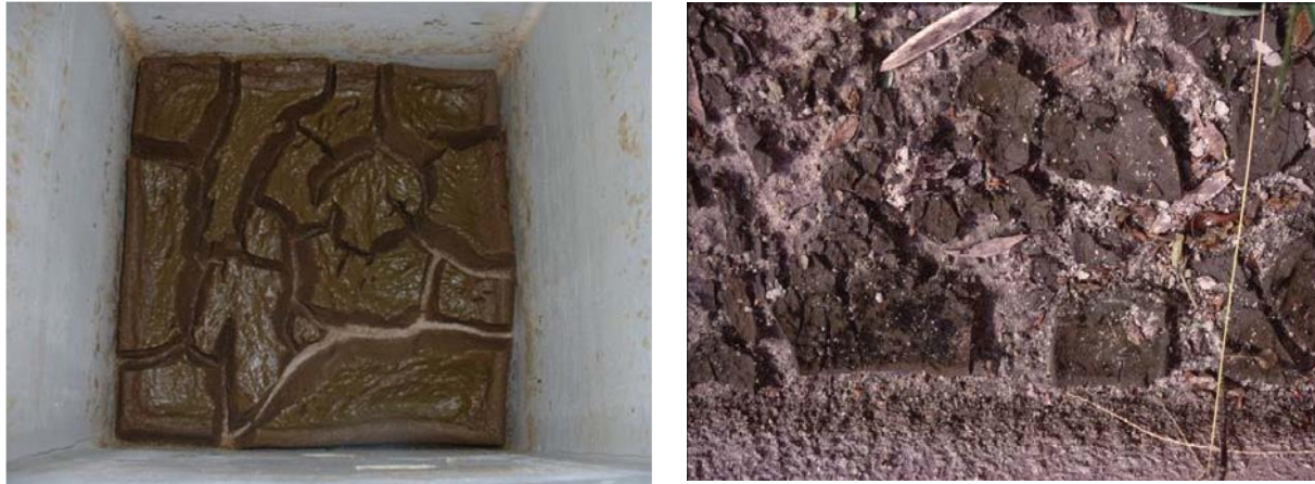
Figure 8. LCWA NuRF Alum Floc Drying Process
