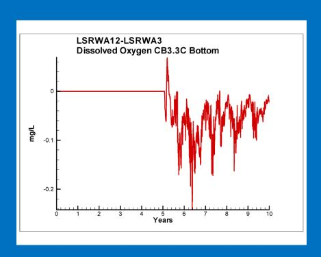
The marginal effect of scour on DO is 0.1 to 0.2 mg/L in the deep trench where DO is critical.
