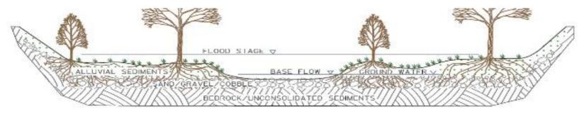
FR-RSB Floodplain Restoration-Raising the Stream Bed is a restoration approach where incised or degraded stream channels are filled with native materials to elevate the stream invert, thereby increasing the annual stream runoff volume diverted into the floodplain.
