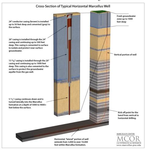
When drilling an unconventional well, operators begin by drilling a vertical wellbore from 5,000 to 9,000 feet into the shale rock. As the vertical wellbore is drilled, various diameters of steel pipe called "casing" are cemented into place in the wellbore. This casing protects groundwater aquifers from pollutants inside the well and helps to stabilize the wellbore as the operator drills farther into the subsurface. The casing also keeps surface water and other geological
