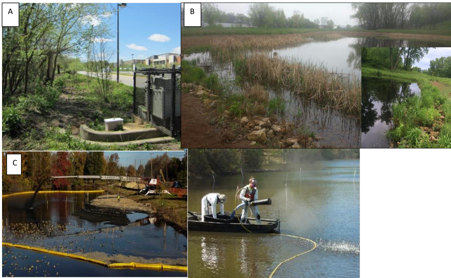
Figure 5. Images of mitigation approaches including watershed BMPs documenting A) PCB removal in bioretention cell (Kjellerup), B) Contaminants of Emerging Concern in iron-enhanced sand filter ponds (Keisling), and C) in-stream applications using bioamended granular activated carbon (Ghosh).
