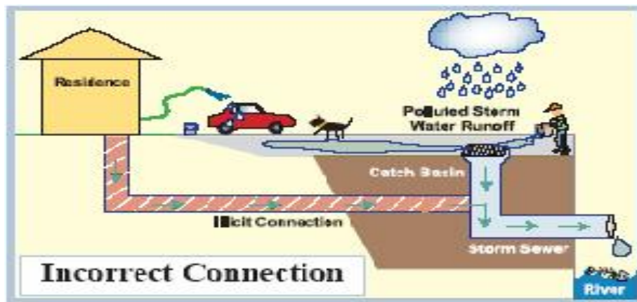
Figure 1. Residential sanitary pipe incorrectly connected to the storm drain system (Photo credit: Kent Count, Michigan, http://www.accesskent.com/Departments/DrainCommissioner/stormwater.htm )
