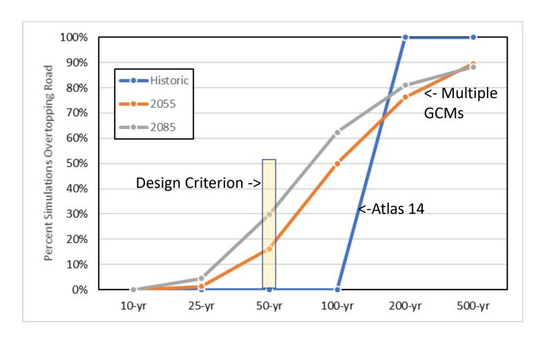
1% slope, 100 ft round culvert, 4.5 ft diameter, 200 cfs design flow, 2 ft freeboard at design flow (matches FHWA Design Guideline 1)
