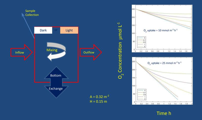
With known leakage, data is fit to a solved differential equation
