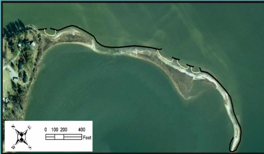
Figure 2. Draft oyster reef sill system for Penniman Spit.
