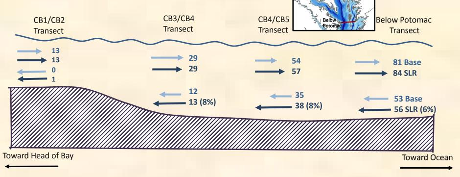
Base = Beta 4 Calibration. SLR = 0.3m Sea Level Rise Scenario representing relative Chesapeake sea level rise from 1995 to 2025. Units in mean kg DO per second ( $m^3/s$ ) for 1991 to 2000 hydrodynamics.
