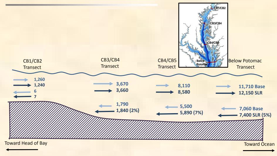
Base = Beta 4 Calibration. SLR = 0.3m Sea Level Rise Scenario representing relative Chesapeake sea level rise from 1995 to 2025. Units in mean cubic meters per second (m³/s) for 1991 to 2000 hydrodynamics.
