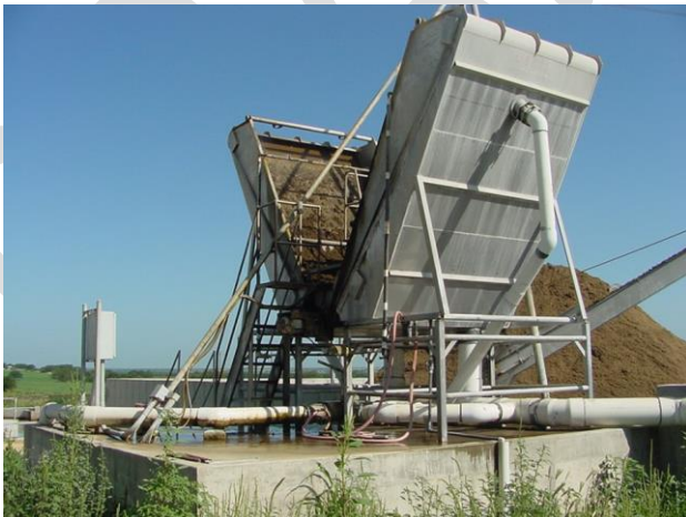
Figure MSLS.2. Dual Inclined Screen Solid Separators in use on a Dairy Farm in Comanche County, Texas (YouTube:OSUWasteManagement).
