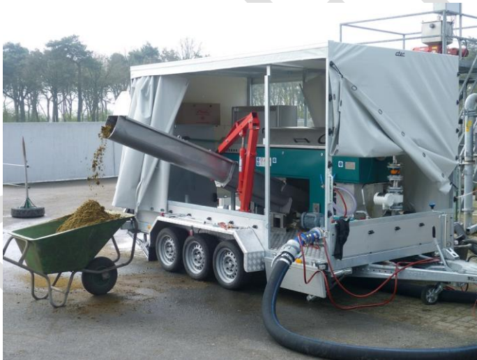
Figure MSLS.9. Decanter Centrifuge (Green and Silver Device on Trailer) being Demonstrated on a Dairy Farm (GEA.com)
