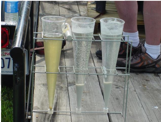
Figure WCT.3. Wastewater from an Alligator Ranch before and after Lime Treatment (YouTube: OSUWasteManagement).
