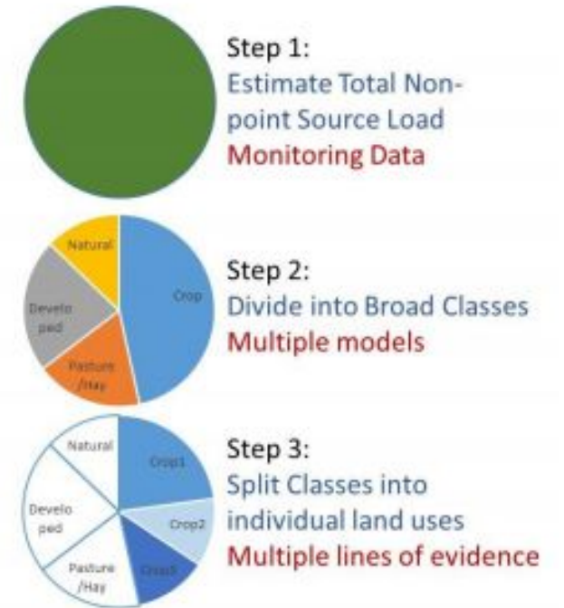
Figure 2-2: Three steps of determining average loads
