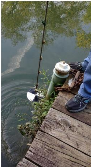
Continuous water quality monitoring station
