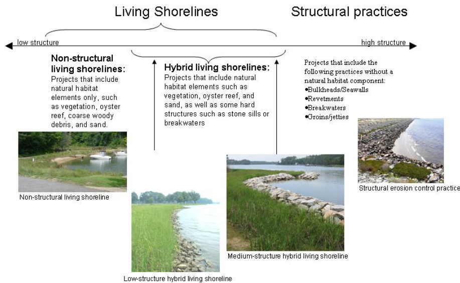
Figure 2. A continuum of shoreline management practices that is based on the amount of hard shore armor structure used.
