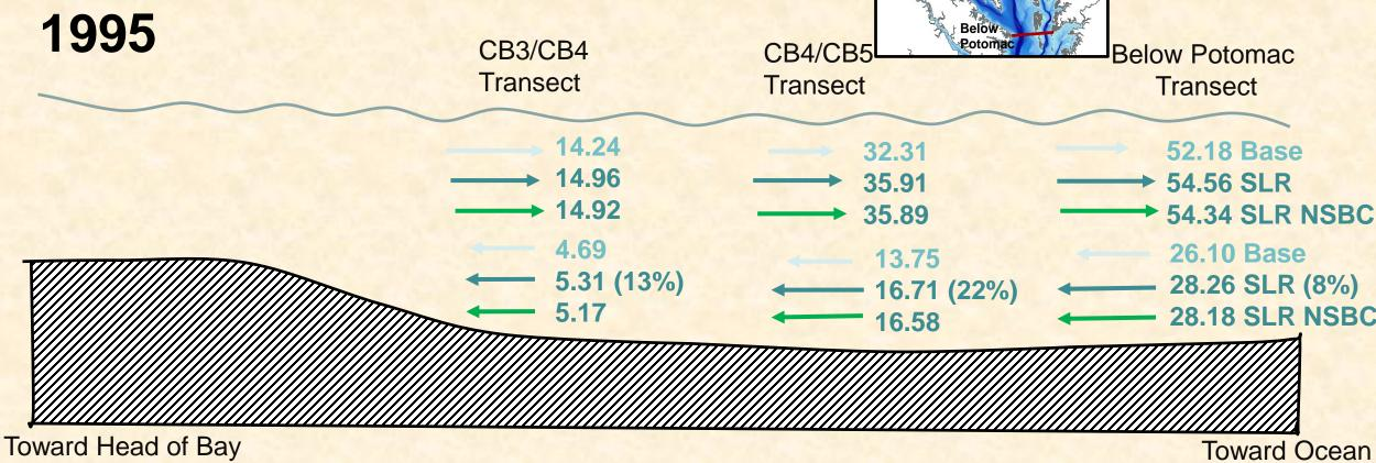
Base = Beta 4 WQSTM, SLR = 0.5m representing relative Chesapeake sea level rise from 1995 to 2050. Units in mean kg DO per second (kg/s) for summer (Jun-Sept) 1993 to 1995; NSBC: No Salt Boundary
