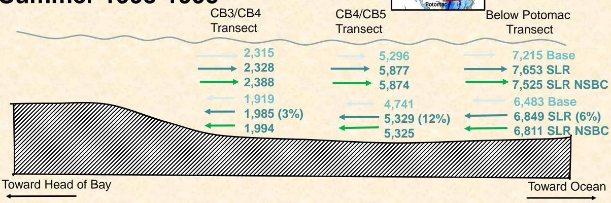
Base = Beta 4 WQSTM, SLR = 0.5m representing relative Chesapeake sea level rise from 1995 to 2050. Units in mean m<sup>3</sup>/s for summer (Jun-Sept) 1993 to 1995; NSBC: No Salt Boundary Change.
