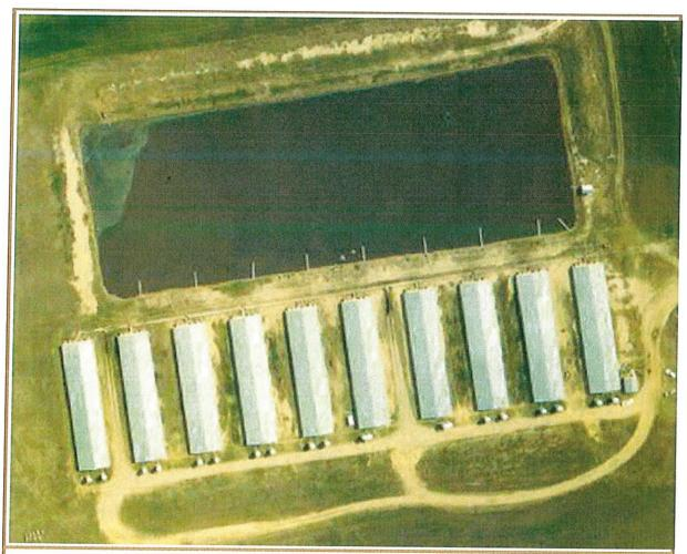
In this large facility, there are two grain bins per building - either for capacity or to facilitate the various rations used in modern swine production. Note the size of the liquid-waste storage pit. Image courtesy of USDA, NRCS.
