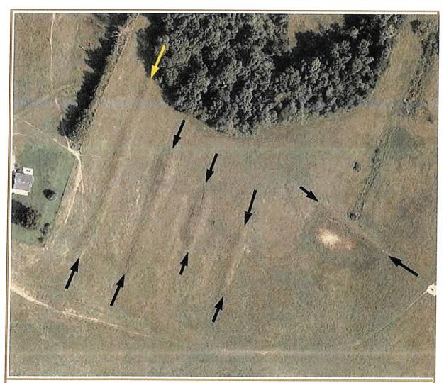
Water-sediment control structures (arrows) in Lauderdale County, Tennessee. Note the minor watercourse that is "interrupted" by these structures. The upper (i.e. left) four structures appear to create very narrow basins, but the lower (i.e. right-most) structure clearly impounds a sizable detention basin. Image courtesy of USDA, NRCS.
