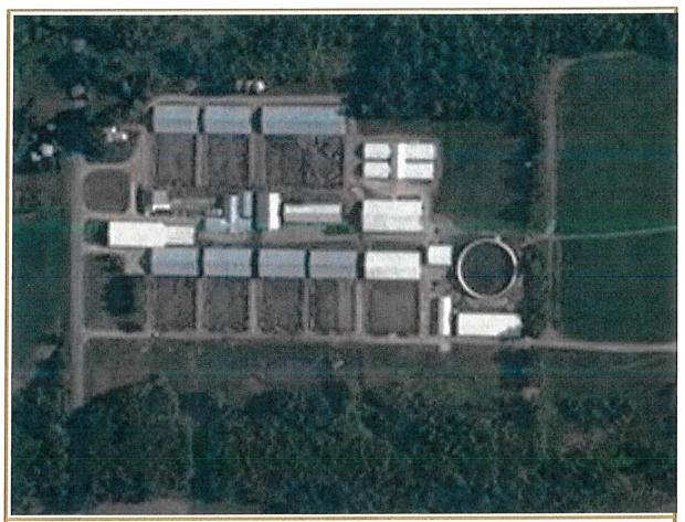
The circular feature at the right-center is a liquid-waste storage pit. Image courtesy of USGS.
