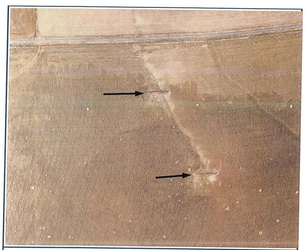
Water-sediment control structures (arrows) in Gilliam County, Oregon. Note the minor watercourse that is "interrupted" by these structures (flow is toward the top of this image). The width of the lighter soil areas immediately up-gradient from the structures indicates how effective they are in creating a sediment trap and water detention basin. Image courtesy of USDA, NRCS.
